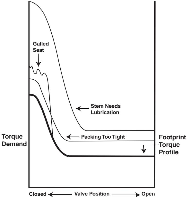
**Opening Torque Characteristics of a Typical Wedge Gate Valve**
