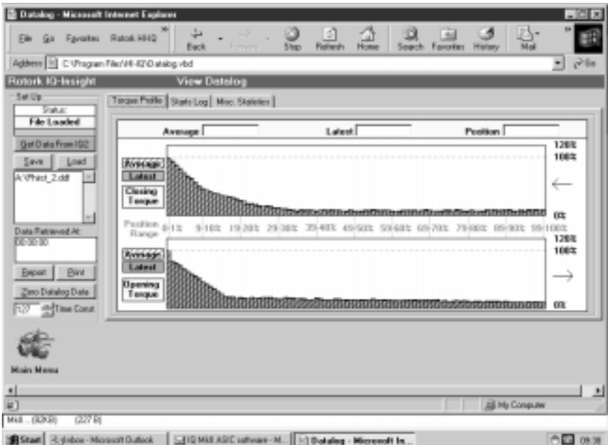
Figure 3. Rotork IQ actuators can gather continuous torque and positioning information. Above is an IQ torque profile using IQ-Insight™ software.
