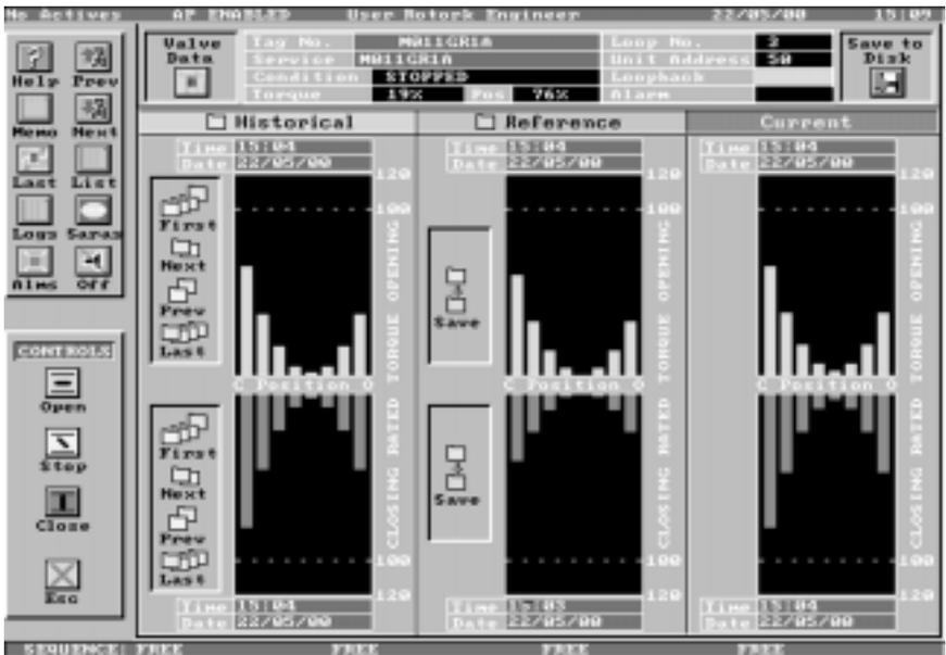
Figure 2. Rotork PakVision and InVision software take data from the IQ actuator via the PakScan system and display it as easy-to-read bargraphs.
