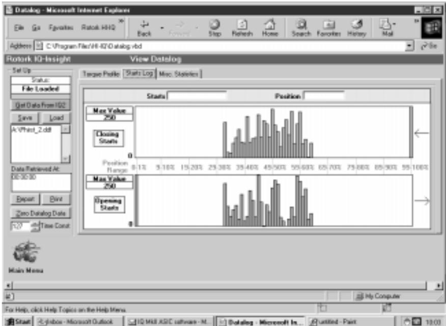
The above image is a view of a Rotork IQ-Insight screen showing frequency of operation data.
